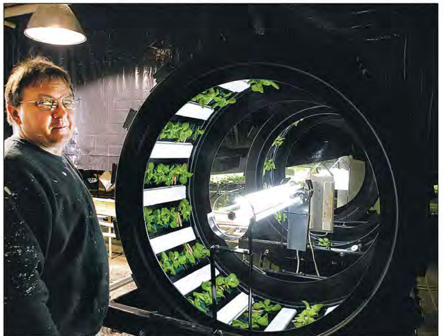
Above: Joe Heineman grows lettuce in a rotating cylinder called Omega Garden. Lights of 600 watts were replaced with 100-watt lights with no discernible growing differences.
